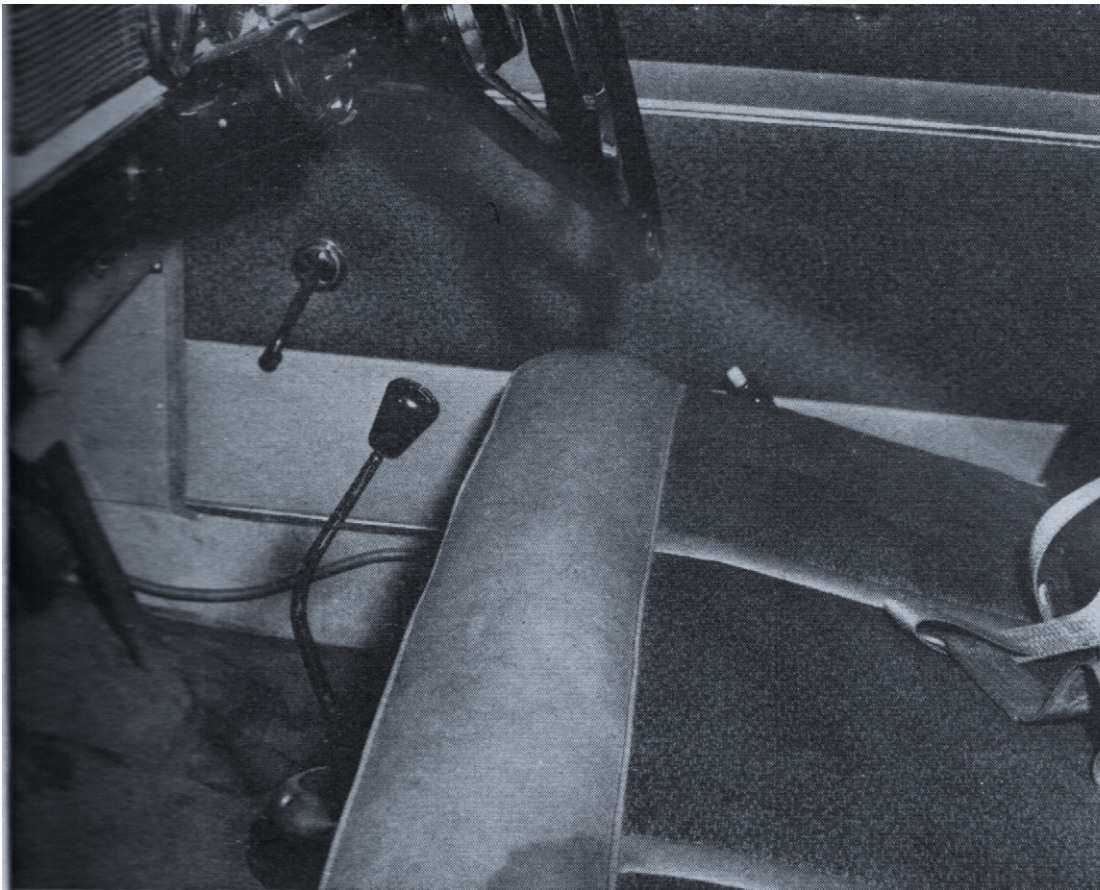
The four speed gearbox and remote control from the Morris Major can be adapted to fit the Freeway, but care is needed in its use.
