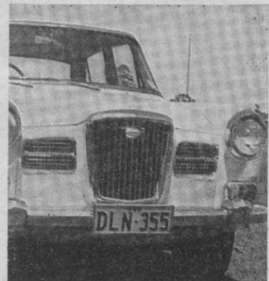
Visible changes are limited to a repositioning of the bumper overriders. Following a time honoured practice the Wolseley insignia is lit with the parking lights.
