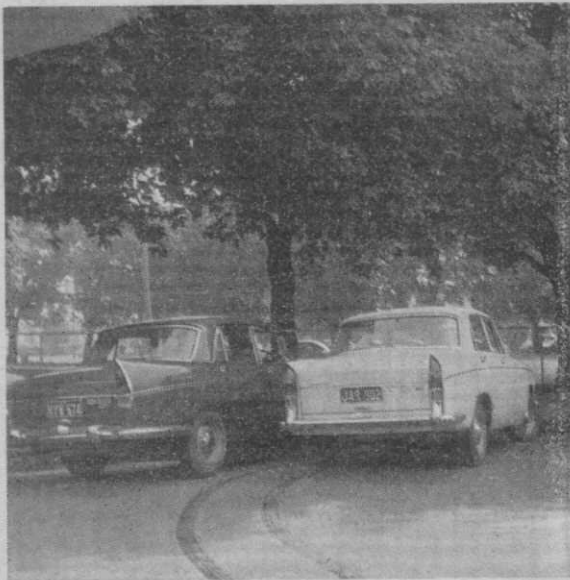
Most noticeable of the external body changes is the reduction in tail fins. Over riders now form part of the tail lights. A central jack point is located at each side of the car.
