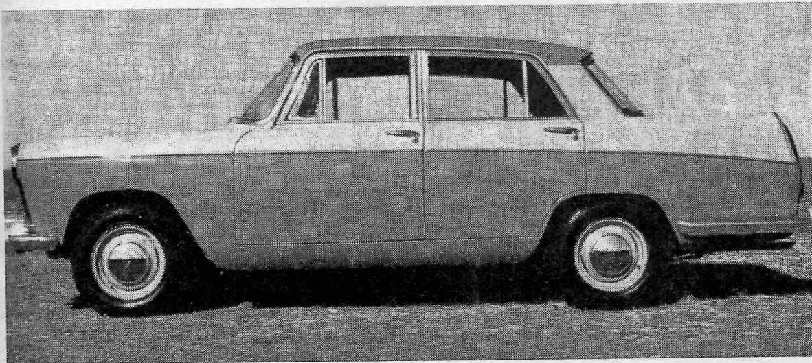
Profile of the Freeway shows the slightly finny treatment of the rear, also how two tone color scheme has been arranged. Wheelbase is an inch longer than A/60's.
