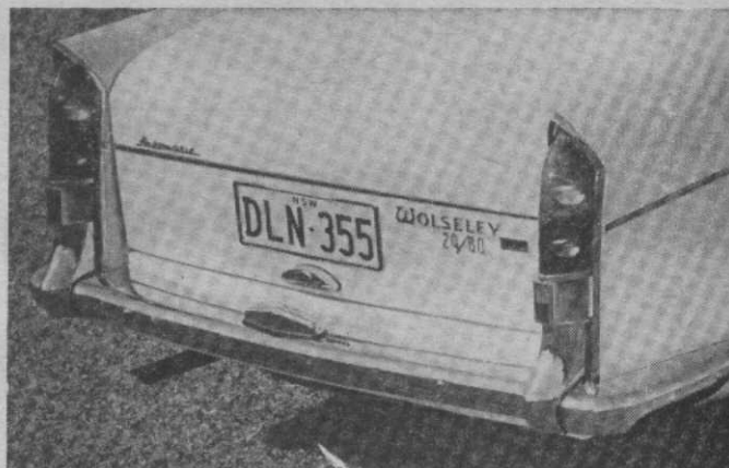
Big clue to the Mk II is the rear. Changes are reshaped tail-lights, trimmed-down fins, altered bumper bar, rewritten "automatic" emblem, and small "Mk II" bezel next to name. However, outline is unchanged.
